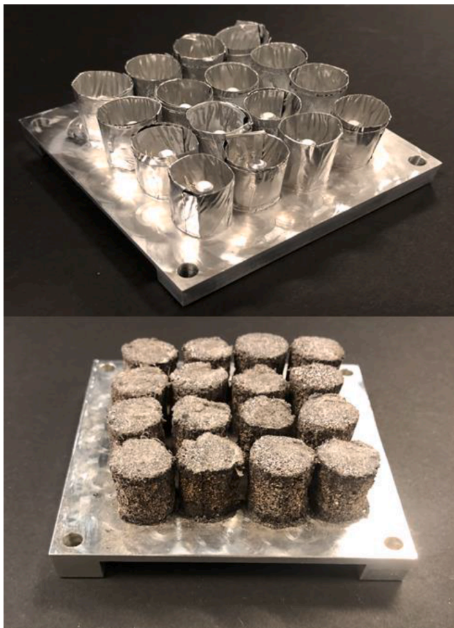
Fig. 2. PF-HMX coated with the composite sorbent, silica gel, CaCl 2 , PVA, and graphite flakes.
